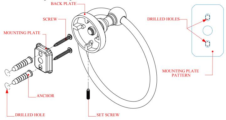
Step 2: Attach Bracket to Mounting Plate
